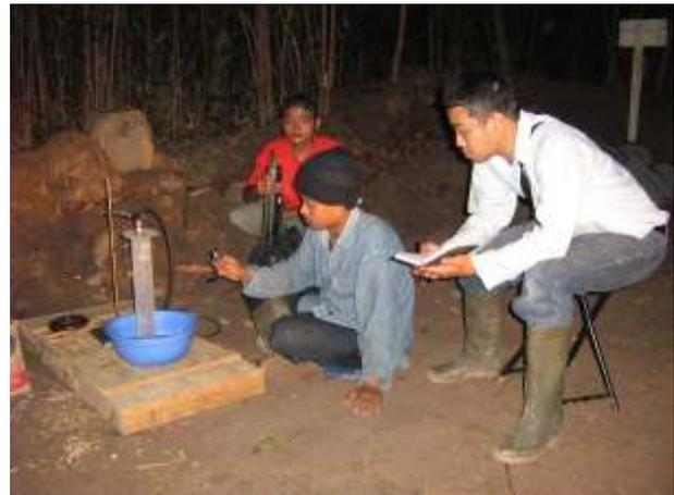
Figure 2. In-situ measurements (Q1) of gas methane content by using simple field equipment in the Bangko Area of PT. Bukit Asam, Tanjungenim, South Sumatera.
