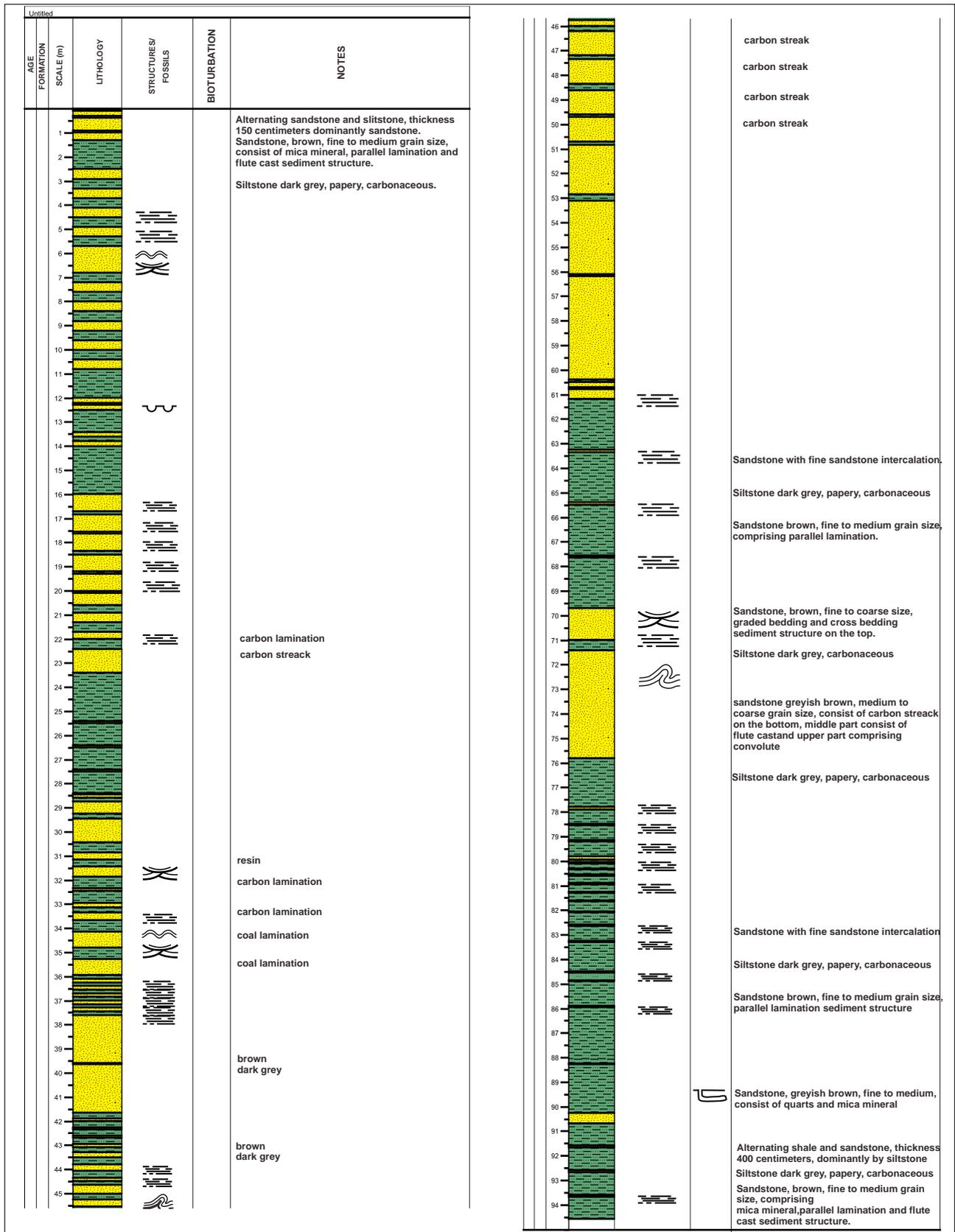
Figure 5. Stratigraphic column of Pedawan Formation in Ledo area.
