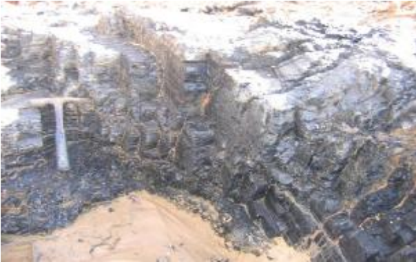
Photo 1. Coal seam showing brownish to black streak, dark grey to black colour, with some of subchoncoidal fractures.
