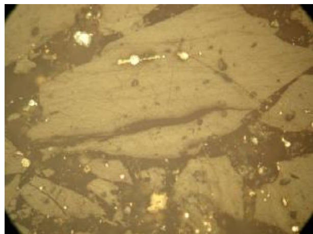
Photo 3. Microphotograph of telocollinite within the coal seam in the Kuansing region (Reflected light): magnification x 200 Sample: 06 MH 47A.
