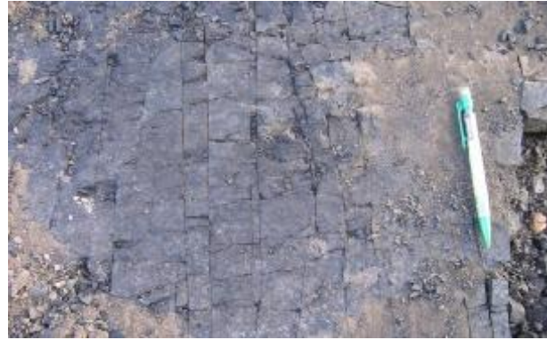
Photo 2. Well developed face cleats in Manunggal Inti Artamas Coalfield.
