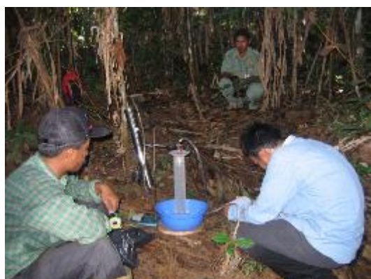
Photo 7. In-situ measurement (Q1) of methane gas, by the Mengkua River, in the Hulumengkua/ Karangjering region, using simple field equipment.
