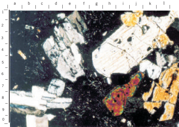
Figure 5. Andesite showing a porphyritic with phenocrist of plagioclase (d4, b8) orthopyroxene (i2, h4, k7) and olivine (h8) set in groundmass of microlith of plagioclase and pyroxene, and glass. Sample 05PDG53A.
