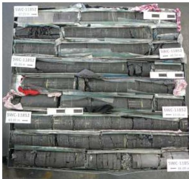
Figure 2. Core of borehole 11852 from the Mulgrave Pit, South Walker Creek.
