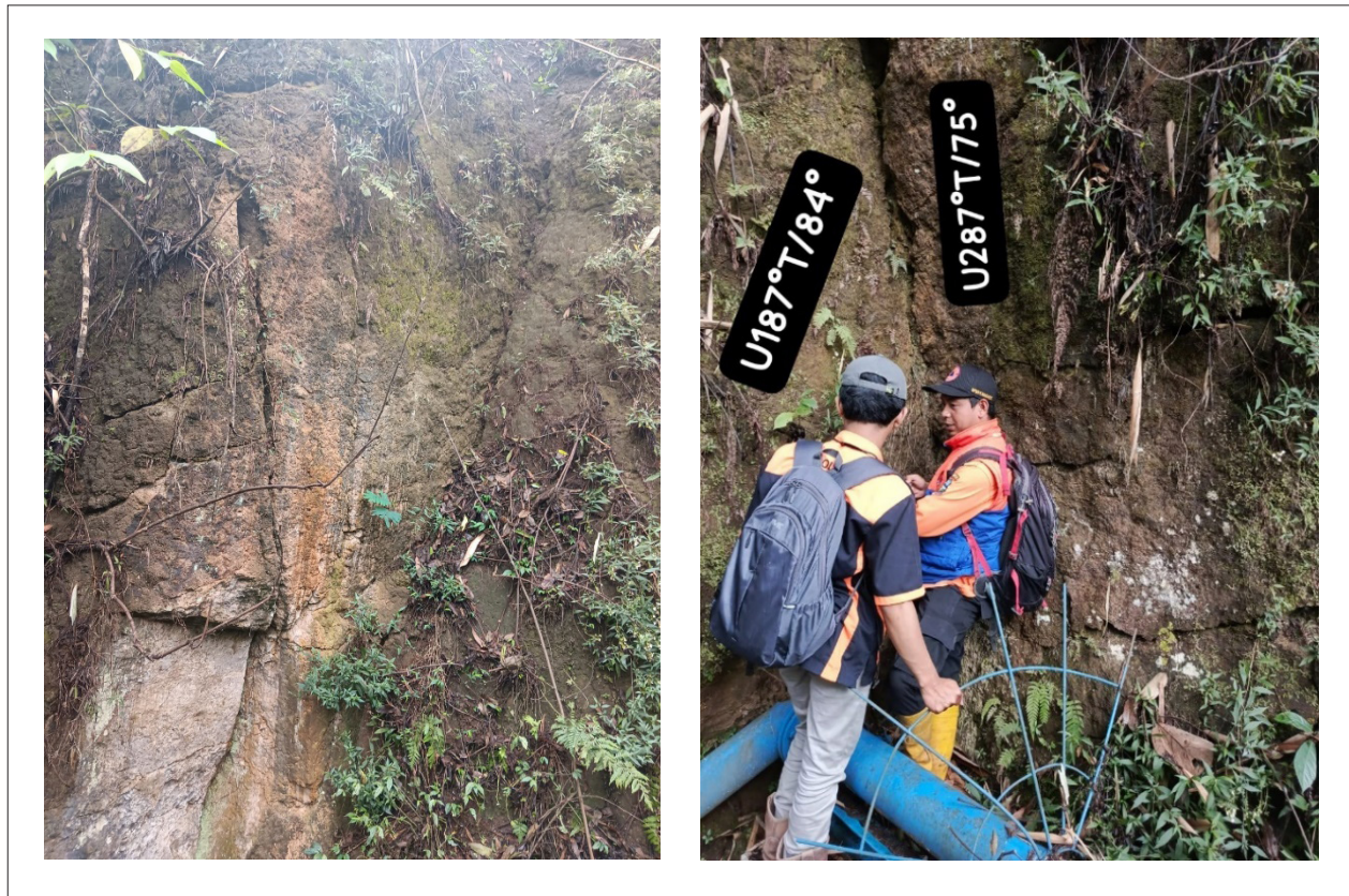
Figure 16. Indication of faults in the form of joints on the Cibongkor Fault Line
